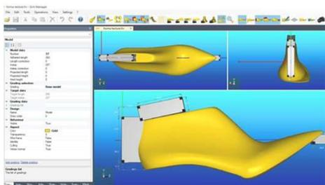
**🇬🇧** *The SetupModel Module of the SLIM 4.0 platform is include. SetupModel allows to add the supports for the clamping on the machine (on toe or heel, for roughing on traditional machinery, or on the top, for finishing on NL-SDF systems).*
