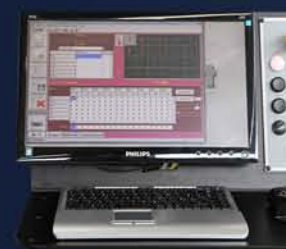
CNC Newlast Easylast 2008 (tempo ciclo assi = 0,5 ms) CNC Newlast Easylast 2008 (time cycle axis =0,5 ms)
